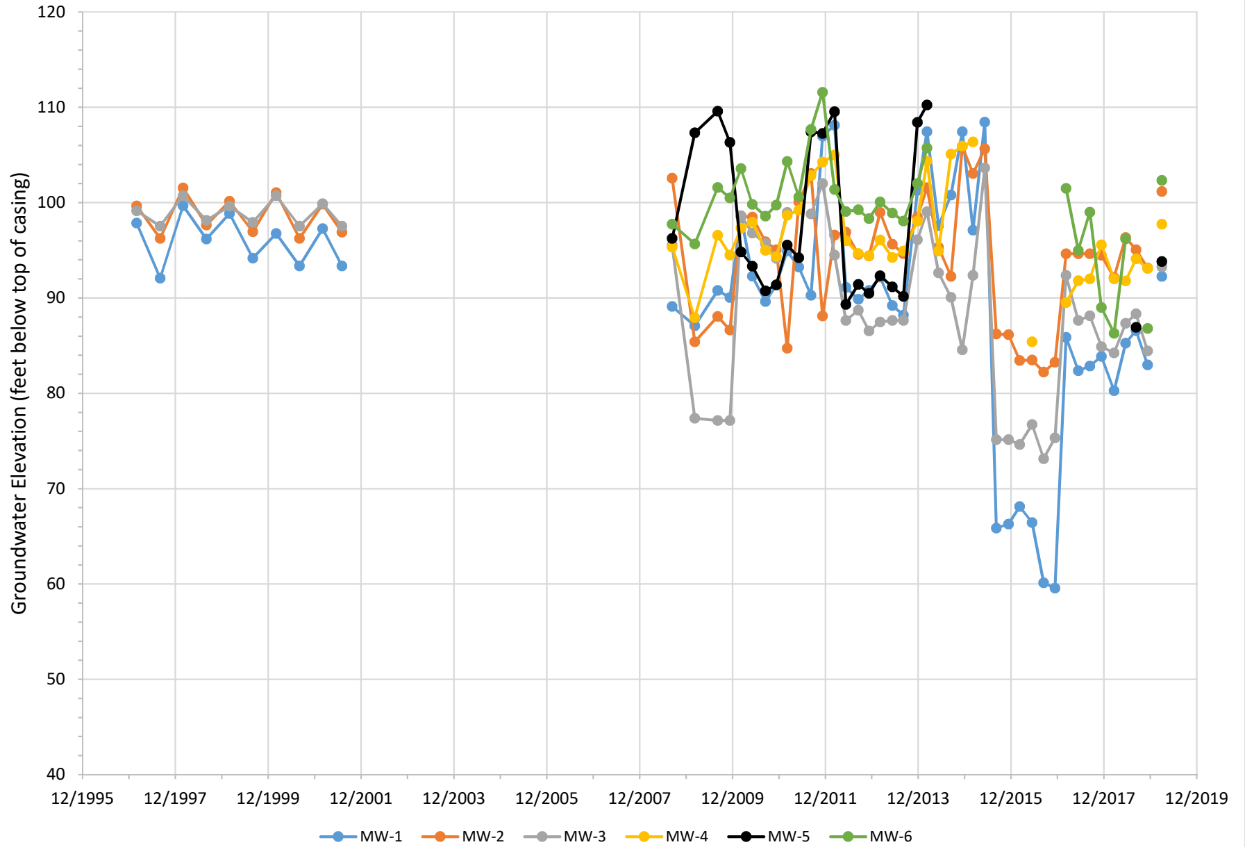
Figure 3. Monitoring Well Groundwater Elevations March 1997 to March 2019
