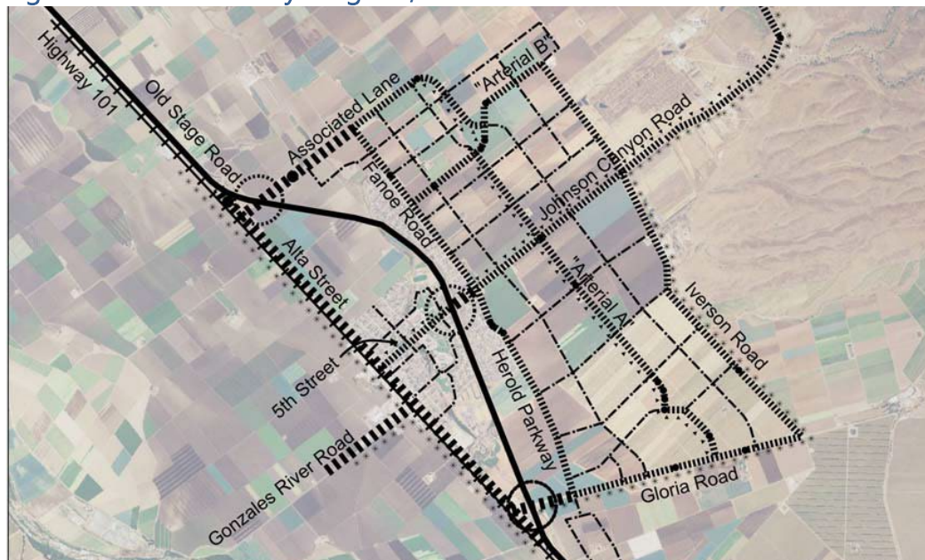
Figure 2.3: Connectivity Diagram, Gonzales General Plan
